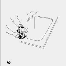
4. Turn the countertop upside down, Apply a light type of caulking compound completely around all edge of sink opening. Stay approximately 1/4" (6.4 mm) from cutout. Use only a 1/8" to 1/4" (3.2 to 6.4 mm) bead of compound. More will make sink difficult to seal. At the same time, prepare several pieces of 2 inch (50 mm) in width marble.
